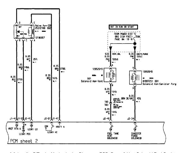
Figure 3.2.1a - II - P/Truck - Mechanization Diagram - EGR, Purge & Vent Solenoid Fuel Canister
